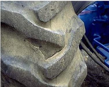
3. Tread is wearing, a few sidewall cracks.
