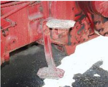
3. Small, narrow, bent, partially removed or modified; rung for step.
