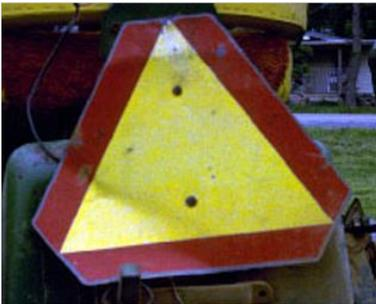
3. Faded, not in correct place; noticeably bent; upside down; partially obstructed; muddy.
