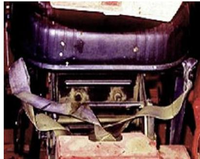
3. Seatbelt straps are properly anchored; straps are oily and/or twisted; straps and buckle difficult to reach.
