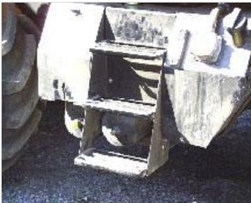
5. Good tread, clean, wide steps; operator's platform is no more than 27 inches high (steps are not required).
