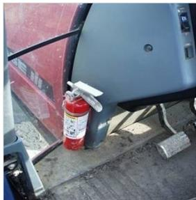
5. ABC type fire extinguisher with at least a 5 pound capacity is mounted on the tractor.
