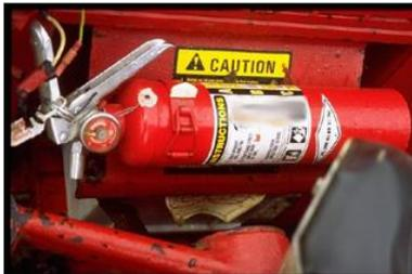
3. BC type fire extinguisher with at least a 5 pound capacity is mounted on the tractor.
