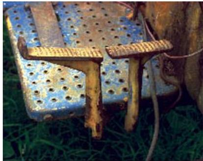
3. Brake locking and setting mechanisms appear partially bent, loose, or out of alignment; difficult to use.
